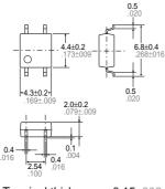
Terminal thickness = 0.15 .006General tolerance:  $\pm 0.1 \pm .004$  Note: For type of connection, see Page 35.
